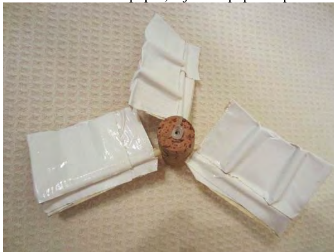
Wind turbine blades made with duct tape and bamboo skewers.
