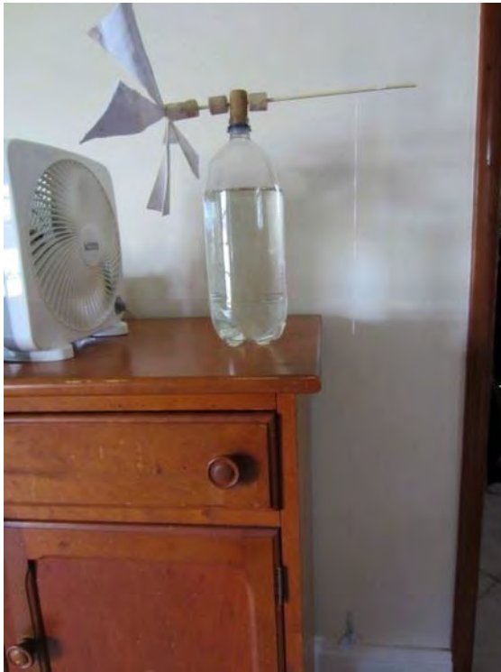
Wind turbine lifts paperclip with washer
