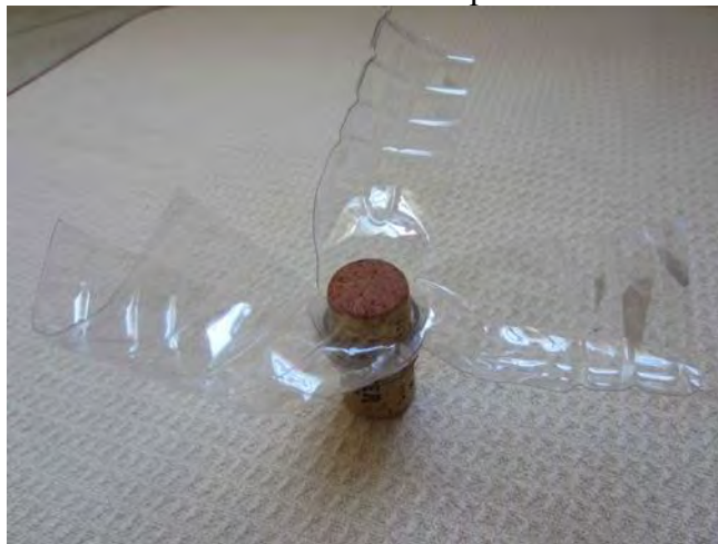
Wind turbine blades made with a plastic bottle.
