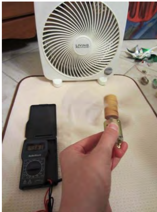
multimeter, box fan and DC motor with turbine attached for testing
