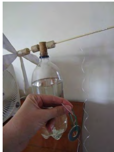
Wind turbine lifts paperclip with washer
